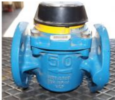
Reference: BPS-184 WATER METER Year: . Brand: ELSTER
