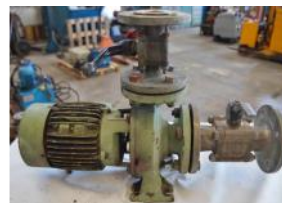
Reference: TOR-068 PUMP CENTRIFUGAL Year: . Brand: CALPEDA
