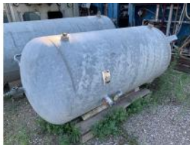
Reference: CCM-028 ACCUMULATION TANK Year: 1992 Brand: X-PAUCHARD
